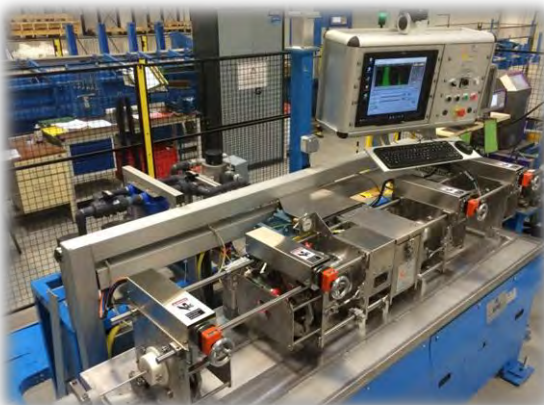
Aeronautic : Bars inspection in special alloys by UT rotating head RotoUTscan
