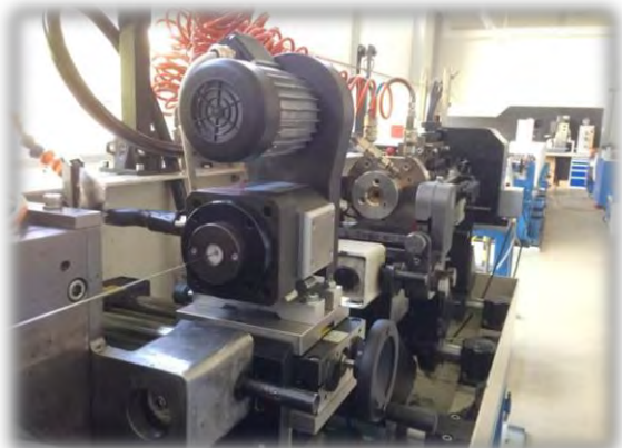
Automotive : Wires inspection by EC rotating head RotoETscan
