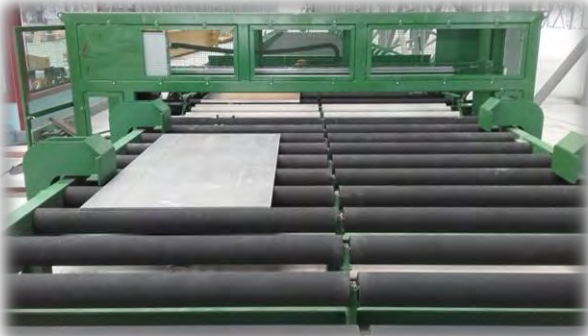
Aeronautic : conductivity measurement on aluminium plate
