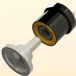
Probe holder for inspection of fuse wheel profile
